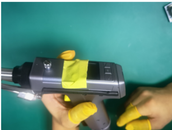
① Use a screwdriver to remove the focusing lens seat screws *2, and then remove the focusing lens seat.
