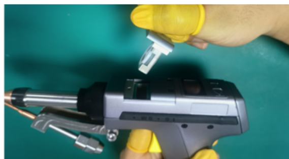
② Remove the protective lens holder
