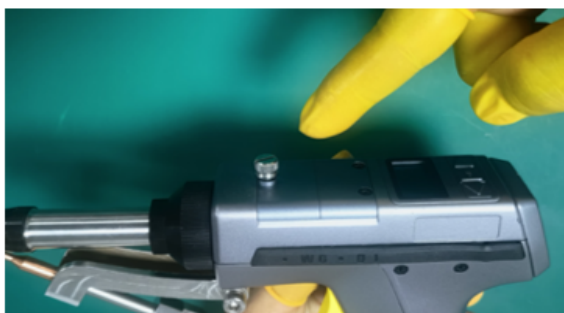
① Unscrew the protective lens screw
