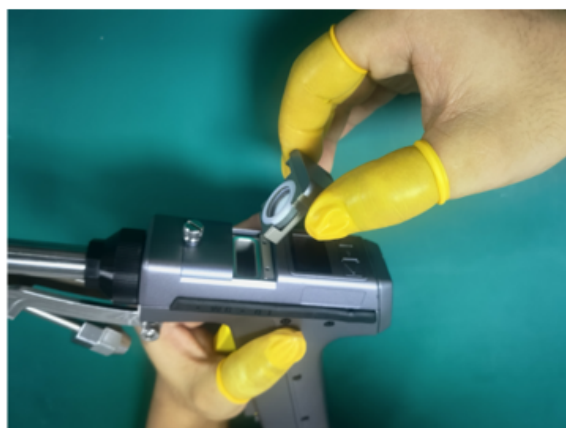
① Use a screwdriver to remove the focusing lens seat screws *2, and then remove the focusing lens seat.
