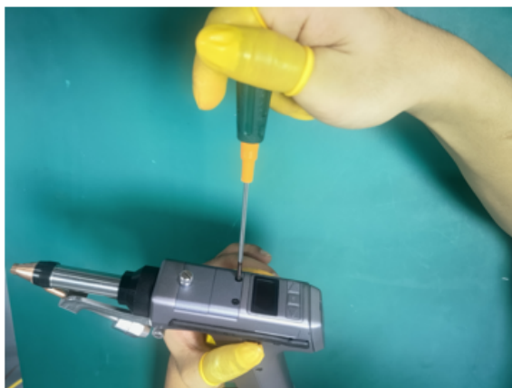
① Use a screwdriver to remove the focusing lens seat screws *2, and then remove the focusing lens seat.
