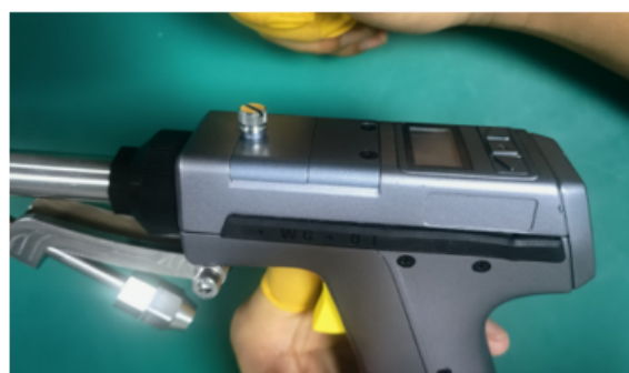
④ Replace the protective lens and install it
