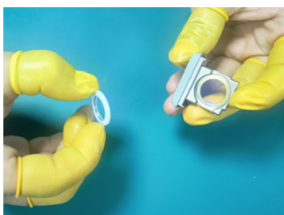
① Use a screwdriver to remove the focusing lens seat screws *2, and then remove the focusing lens seat.
